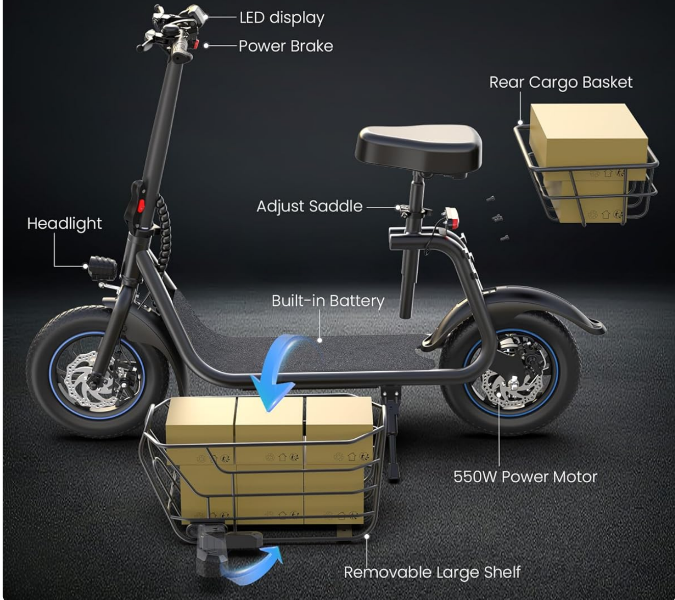
Figure 2.2: Key components of the Gyroor C1S Electric Scooter.
