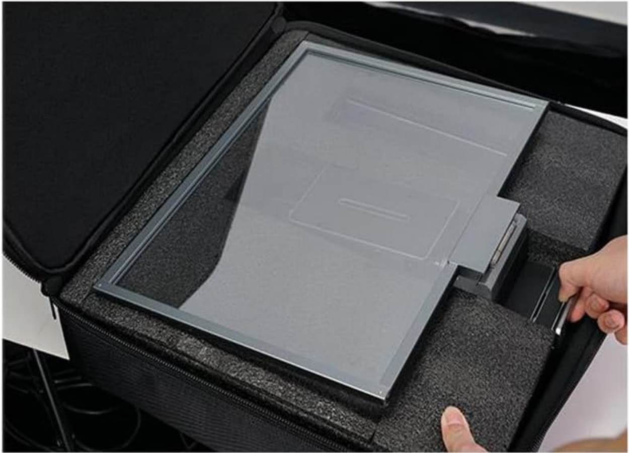
Figure 3.2: Installation or removal of the beam-splitting glass, highlighting its size and careful handling.
