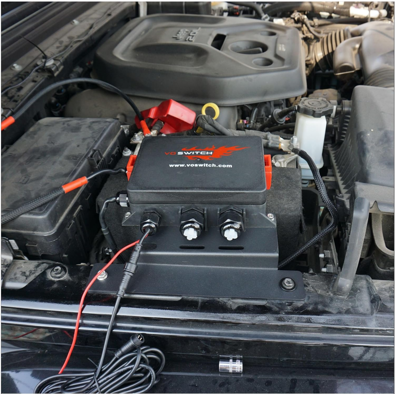
Image: Power Module Installed in Engine Bay
