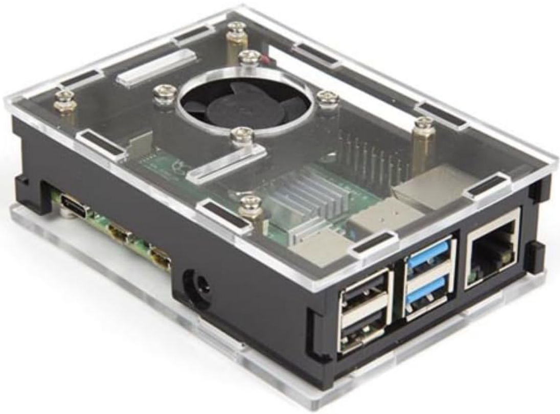
Image 2: Top view of the Raspberry Pi 4 board securely installed within the cooling case, showing the fan and various components.
