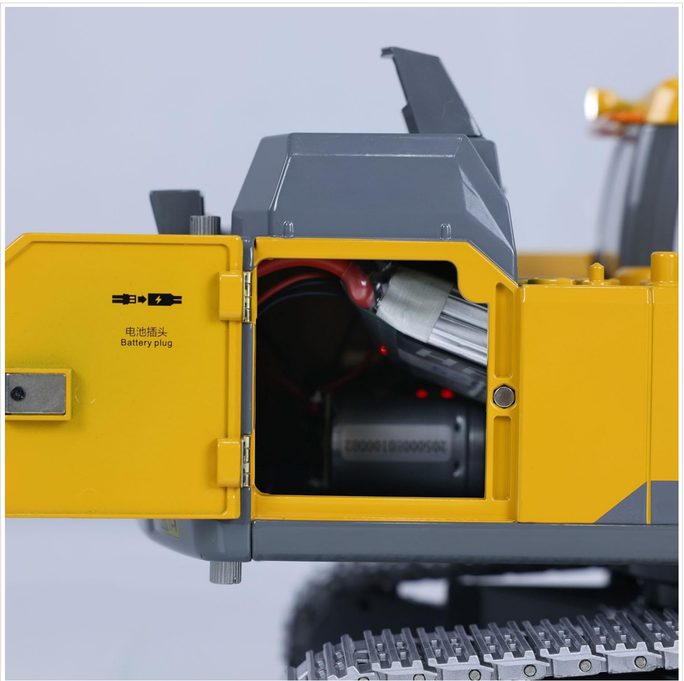
Image 2: Rear view of the excavator showing the open battery compartment with the battery plug clearly visible.
