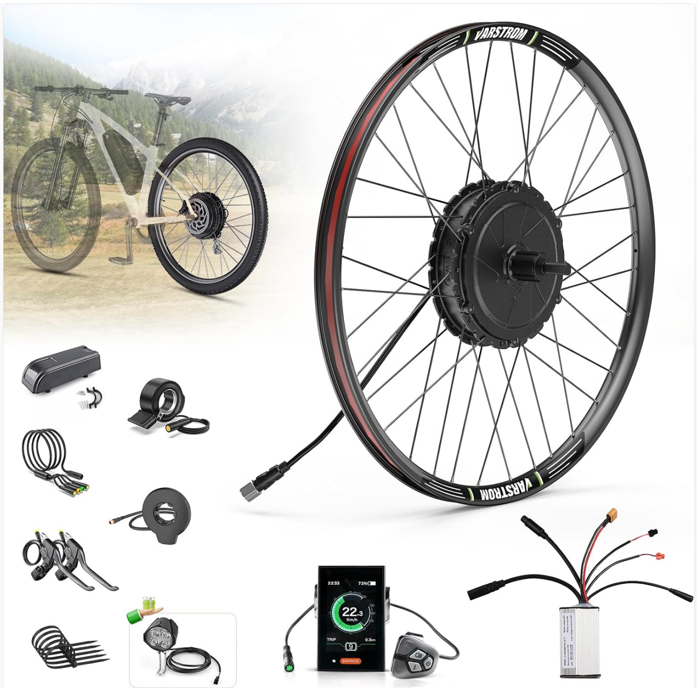
Figure 1.1: BAFANG G0900 Electric Bicycle Conversion Kit components including the rear hub motor, display, controller, brake levers, thumb throttle, PAS sensor, and cables.
