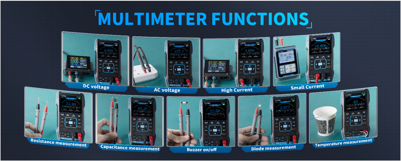
Figure 4.2.2: An overview of the diverse measurement functions available in multimeter mode.
