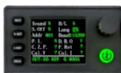
Figure 5.3: Menu interface options for sound, backlight, screen stop, language, device address, baud rate, startup icon, startup output, zero calibration, voltage calibration, and current calibration.
