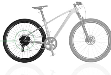
Figure 5.1: Wheel size options and rear dropout measurement for compatibility.
