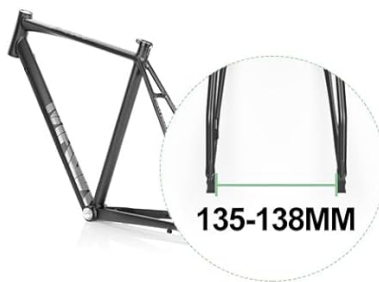
Figure 5.1: Wheel size options and rear dropout measurement for compatibility.
