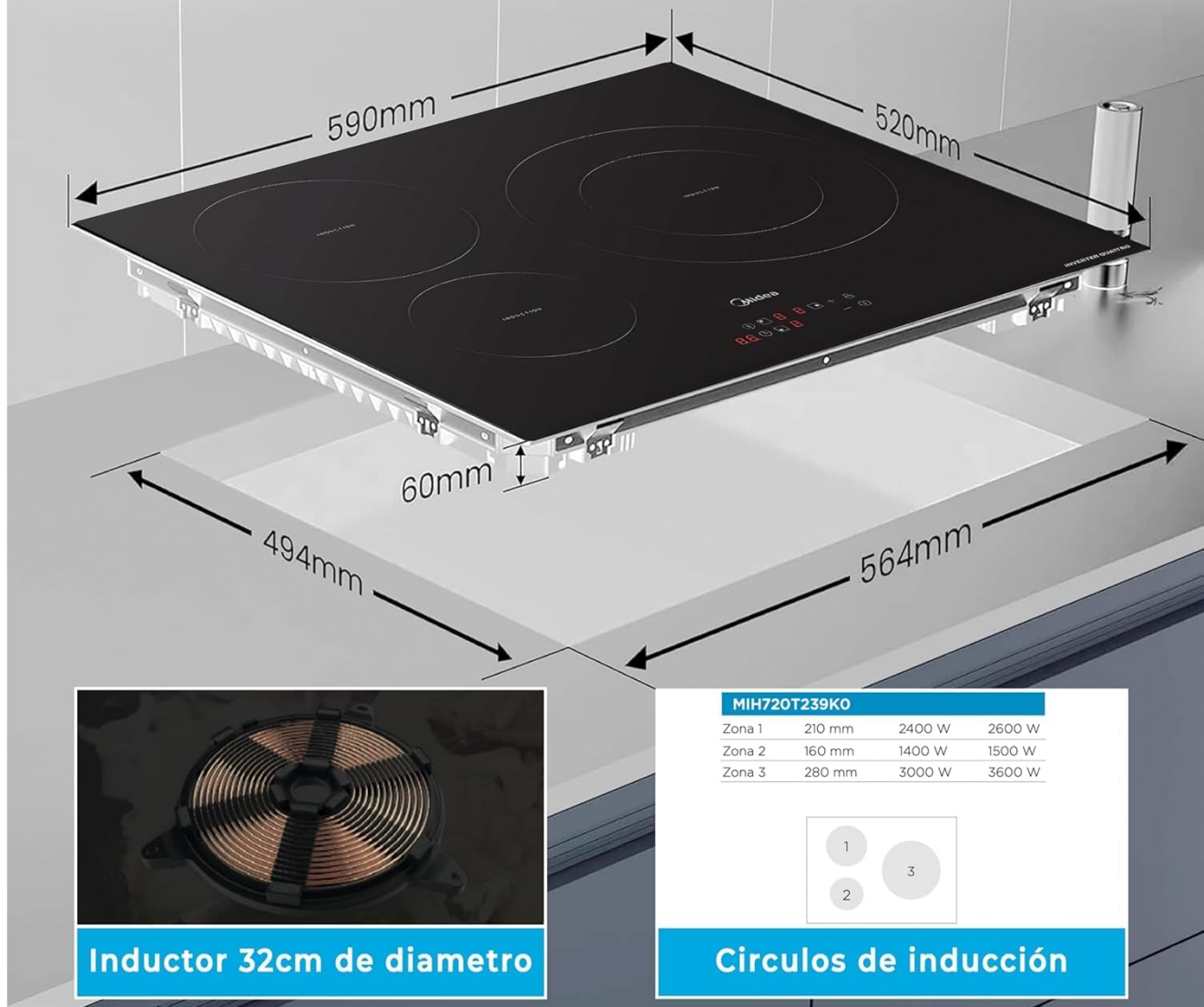
Figure 3.1: Cooktop Dimensions and Zone Specifications. The cooktop measures 590mm x 520mm with a depth of 60mm. It features three zones: Zone 1 (210mm, 2400W/2600W Boost), Zone 2 (160mm, 1400W/1500W Boost), and Zone 3 (280mm, 3000W/3600W Boost).
