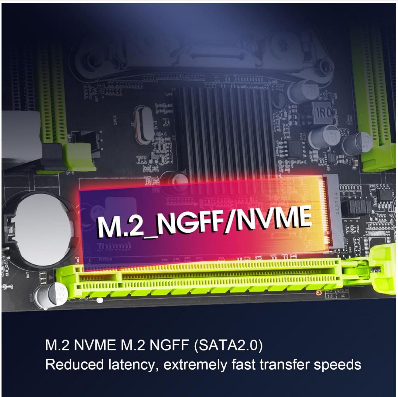
Figure 2.1: M.2 NVME/NGFF Slot for high-speed storage.
