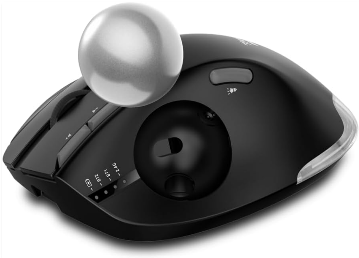
Image: The trackball separated from the mouse, showing the socket for cleaning.
