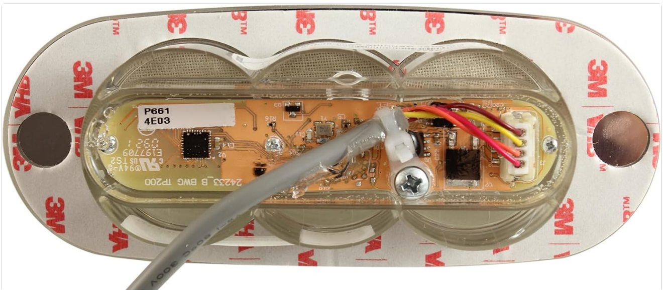
Image 3.2: Rear view of the Balboa Water Group G8425 TP240T Topside Control Panel. This image highlights the internal wiring connections, the circuit board, and the adhesive backing (marked '3M') used for mounting and sealing the panel to the spa shell.
