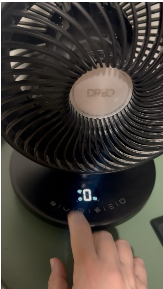
Image: Close-up of the fan's control panel, showing icons for power, fan speed, timer, oscillation, and mute functions.
