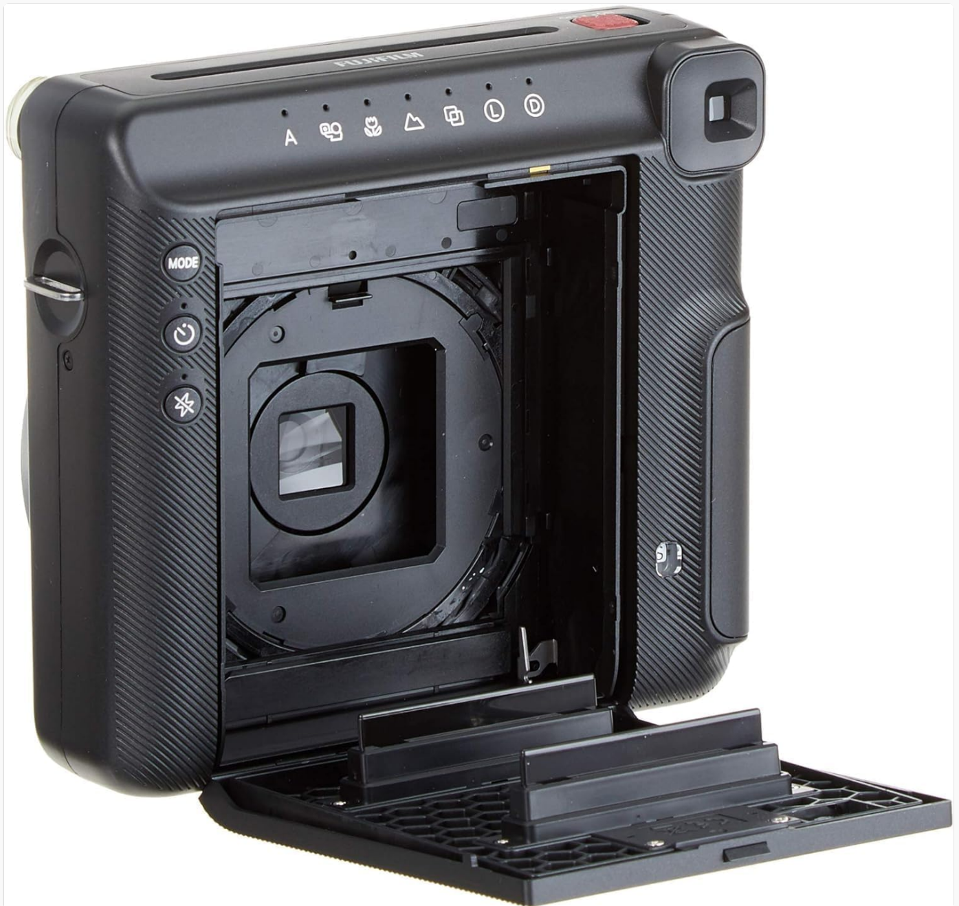
Image 4.1: The Instax Square SQ6 with its film compartment open, ready for film loading.
