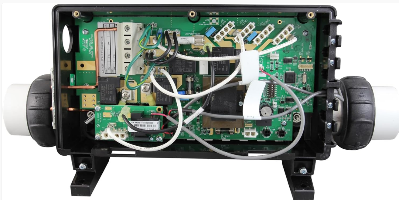
Figure 4.2: Internal view of the Balboa BP100G2 control unit, showing the circuit board, relays, and wiring terminals. This view is for reference during professional installation and troubleshooting.
