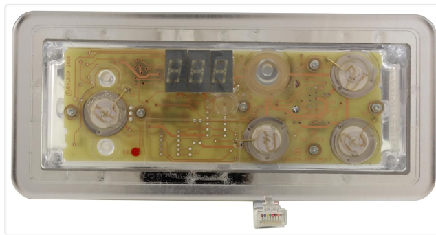
Figure 3: Front view of the VL404 control panel's internal components, showing the display and button locations.
