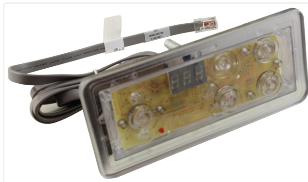
Figure 1: Angled view of the VL404 control panel showing the RJ45 cable connection.
