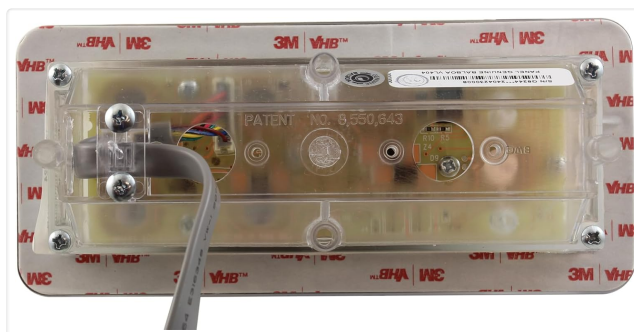
Figure 2: Rear view of the VL404 control panel, illustrating the adhesive backing for mounting.
