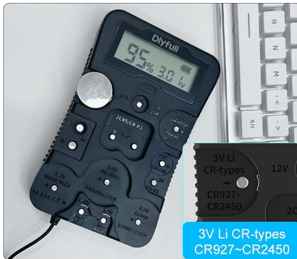
Image: Demonstrations of testing various battery types using the Diyfull B4 tester, including cylindrical, 9V, and button cell batteries.
