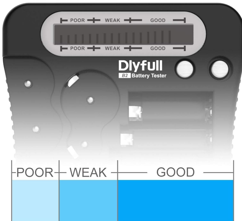
Image: Close-up of the DLYFULL B2-Black's LCD screen, illustrating the "Poor," "Weak," and "Good" indicators for battery health.
