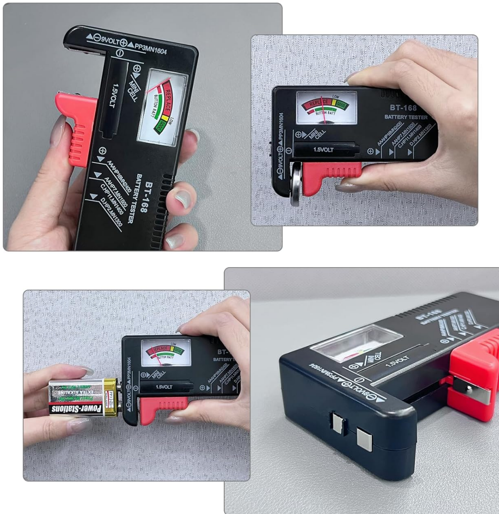
Image: A series of images demonstrating how to test various battery types, including 1.5V cylindrical batteries, 9V batteries, and button cells, using the DLYFULL B1L tester.
