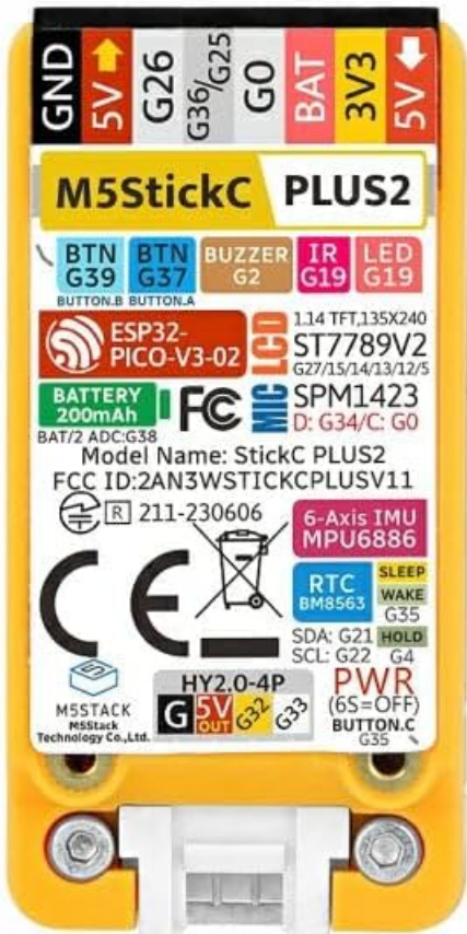
Image: The back panel of the M5StickC PLUS2, showing printed technical specifications including the ESP32-PICO-V3-02 chip, 8MB Flash, 2MB PSRAM, 1.14 TFT display, 200mAh battery, and various sensor details.
