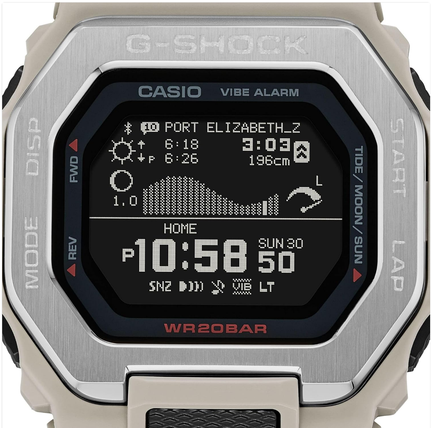
Figure 2: Close-up of the watch face, highlighting the high-resolution MIP LCD. The display shows time, date, tide graph, and other indicators, which are configurable via the G-SHOCK MOVE app after pairing.
