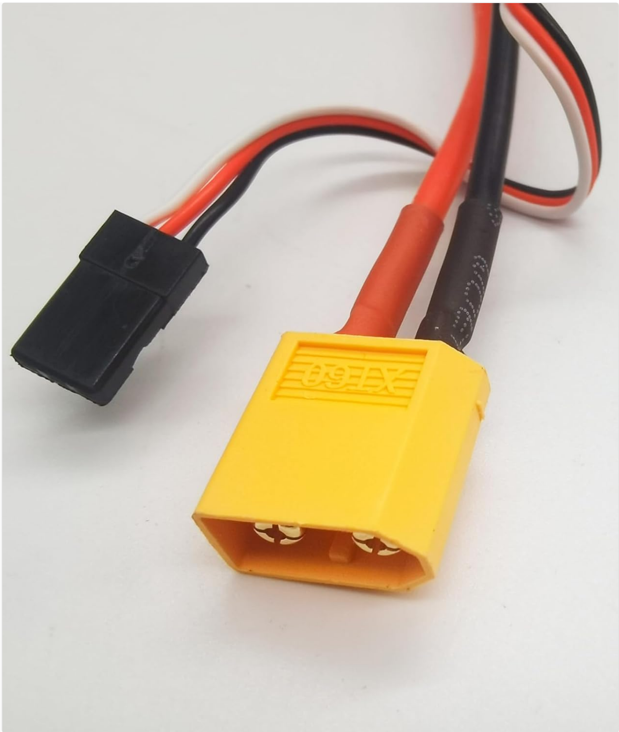
Figure 3.2: Detail of the yellow XT60 battery input connector and the black servo signal connector (JR style) for receiver connection.
