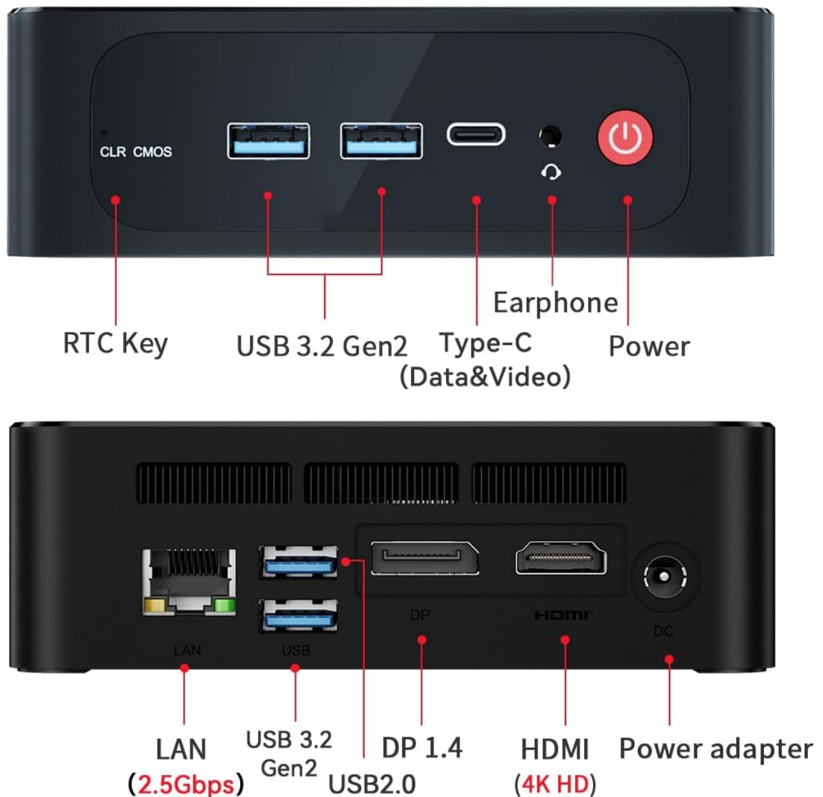
Figure 4: A close-up view of the various connectivity ports on the Beelink SER5 Mini PC, including USB, HDMI, DisplayPort, LAN, and Type-C.
