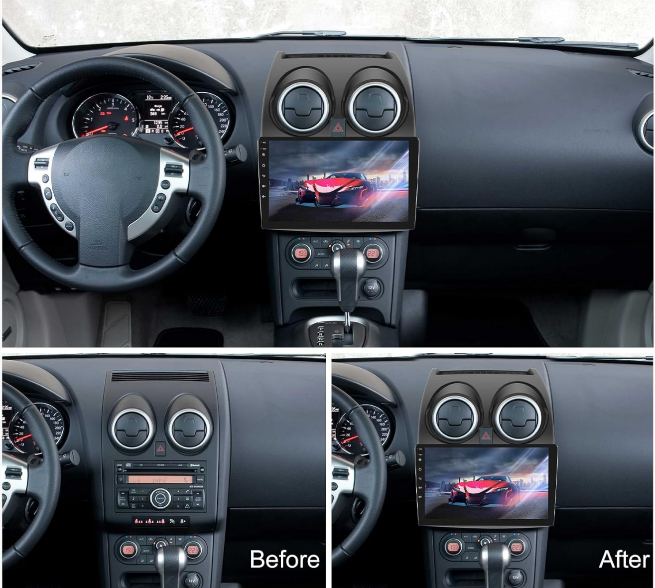
Figure 1.1: Before and after installation of the SIXWIN Autoradio in a Nissan Qashqai J10 dashboard. The new unit replaces the original stereo system, providing a larger display and modern features.
