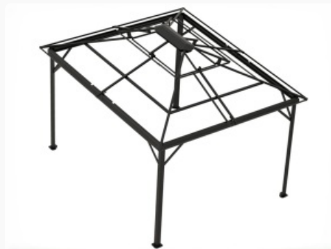
Step 2: Construct the roof frame.
