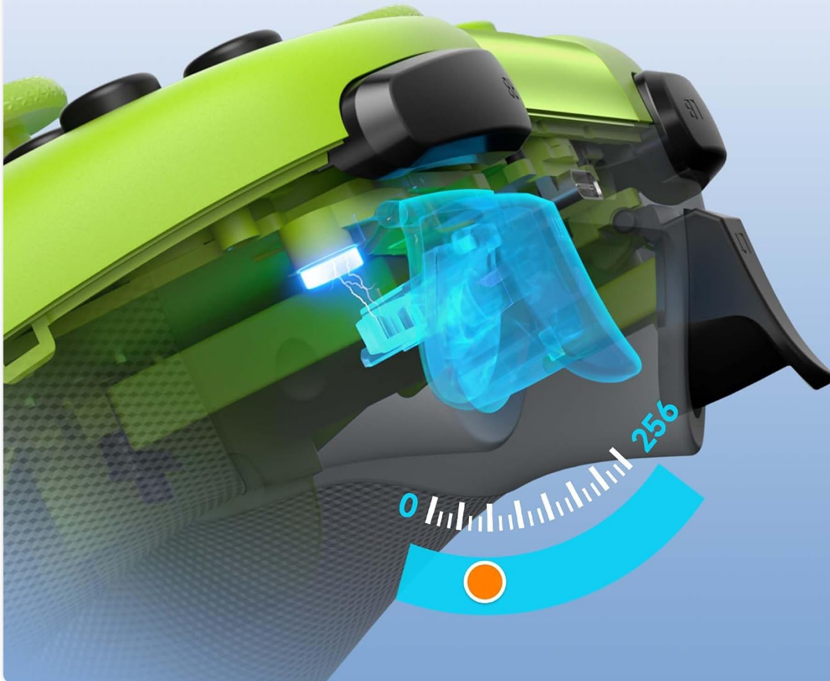
Figure 3.3: Hall Effect Triggers
