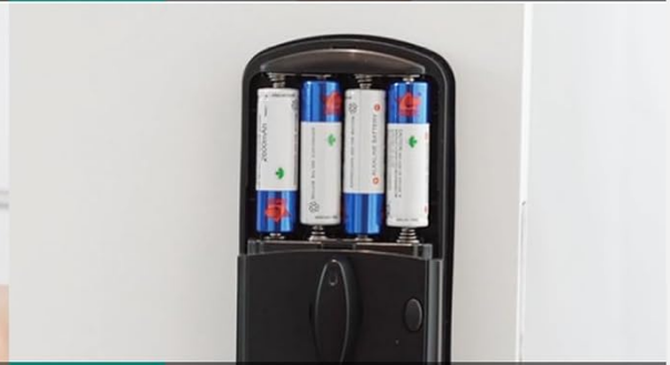
STEP 6 Install the batteries and cover
