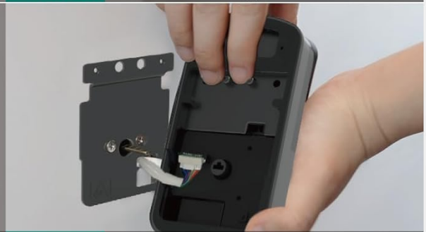
STEP 4 Connect the cable
