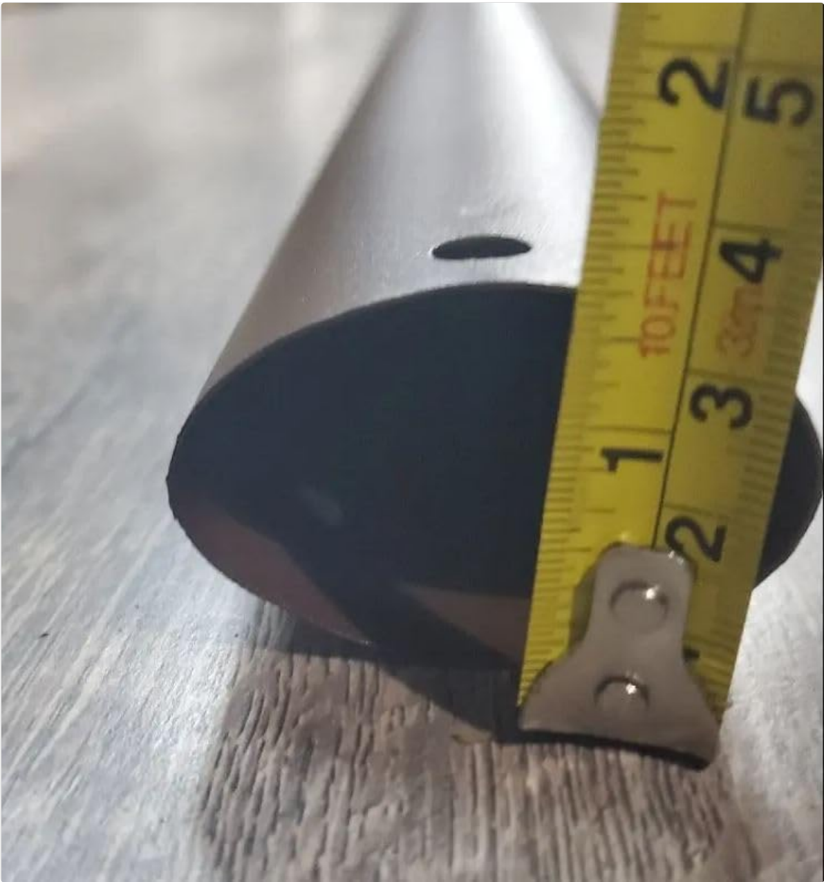
Figure 7.2: The replacement leg being measured for its width, approximately 2 inches.
