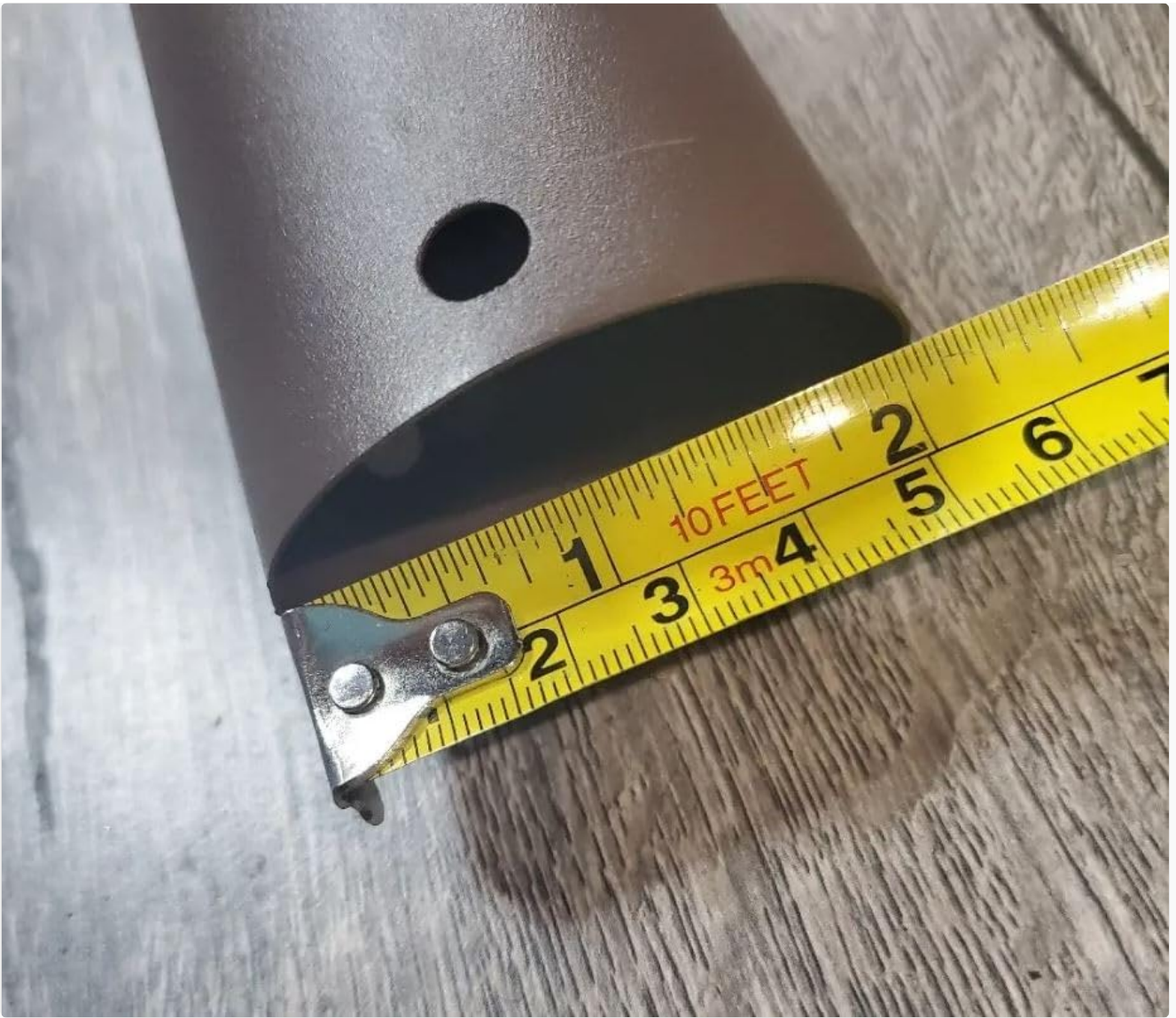
Figure 7.3: The replacement leg being measured for its thickness, approximately 1.25 inches.
