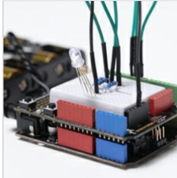
Image: A circuit demonstrating the RGB LED project, showcasing color mixing capabilities.
