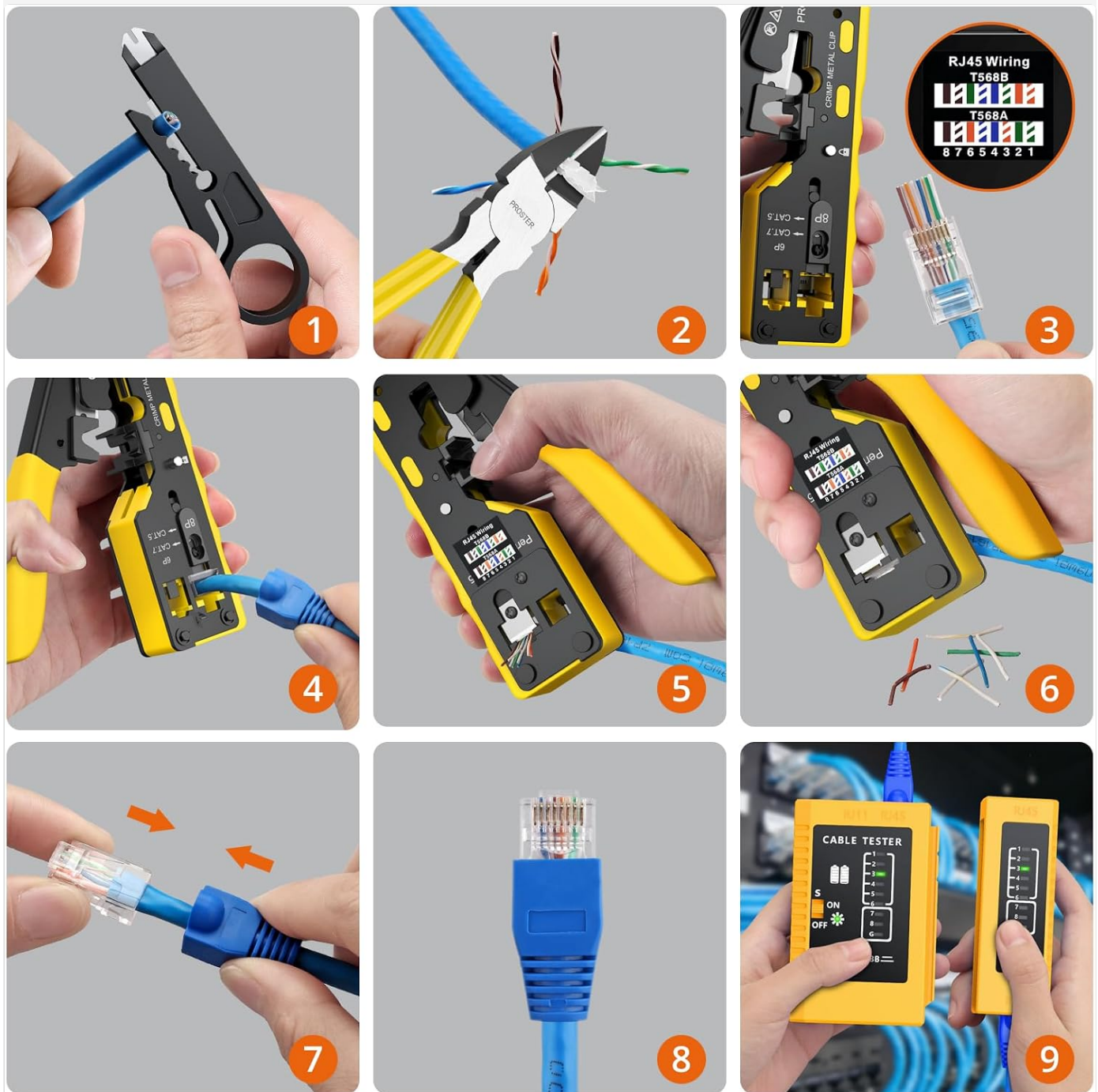
Figure 5: Step-by-step guide for preparing and crimping an RJ45 connector.
