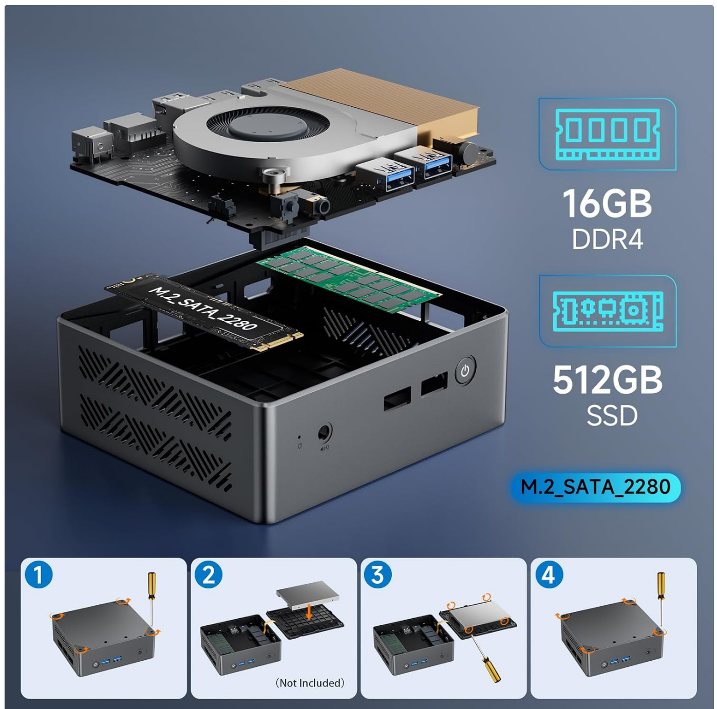
Figure 3.2: Memory and Storage Configuration
