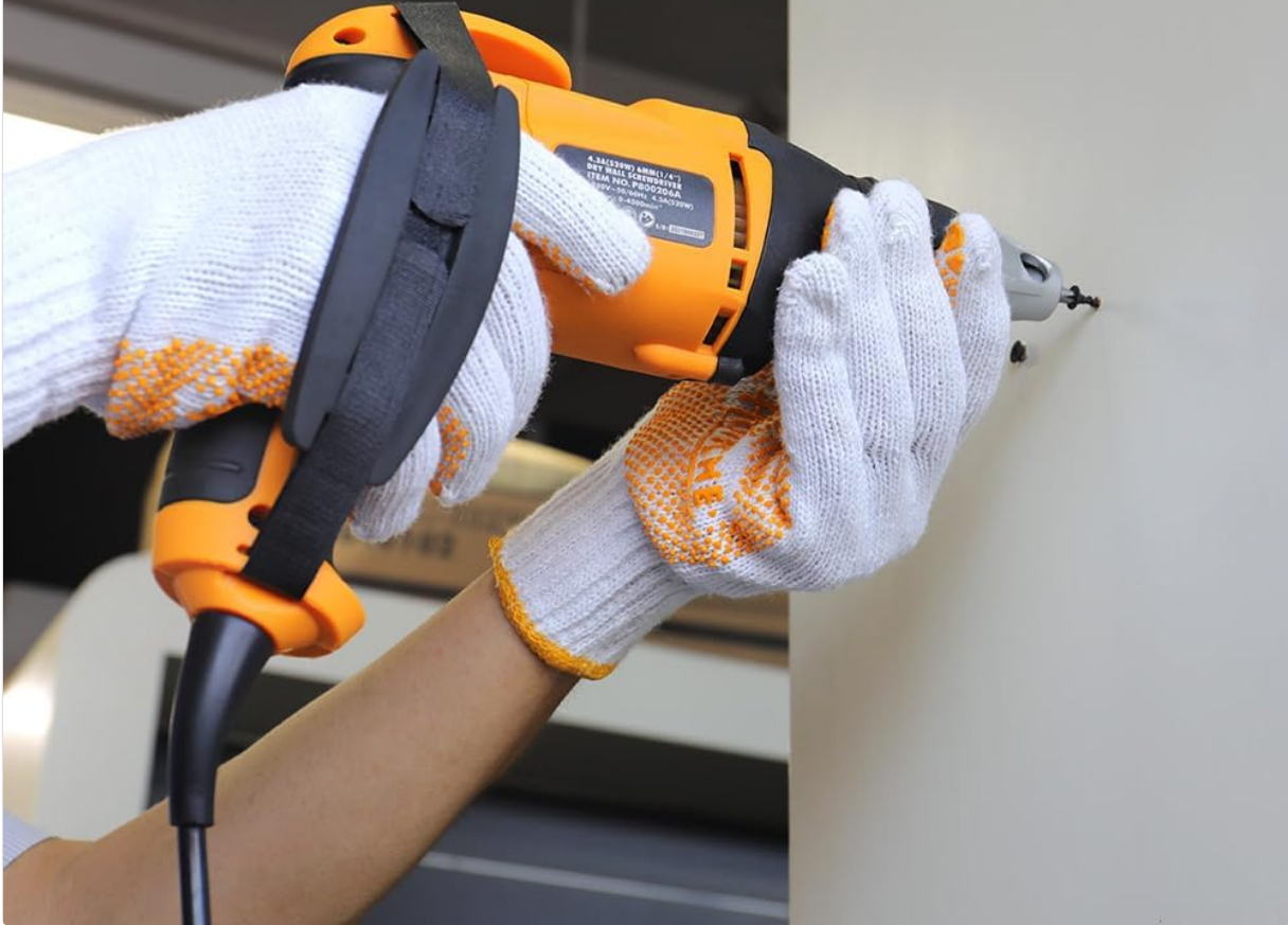
Figure 4.2: Adjusting the screw length by rotating the depth control ring. This allows for precise control over how deep the screw is driven.
