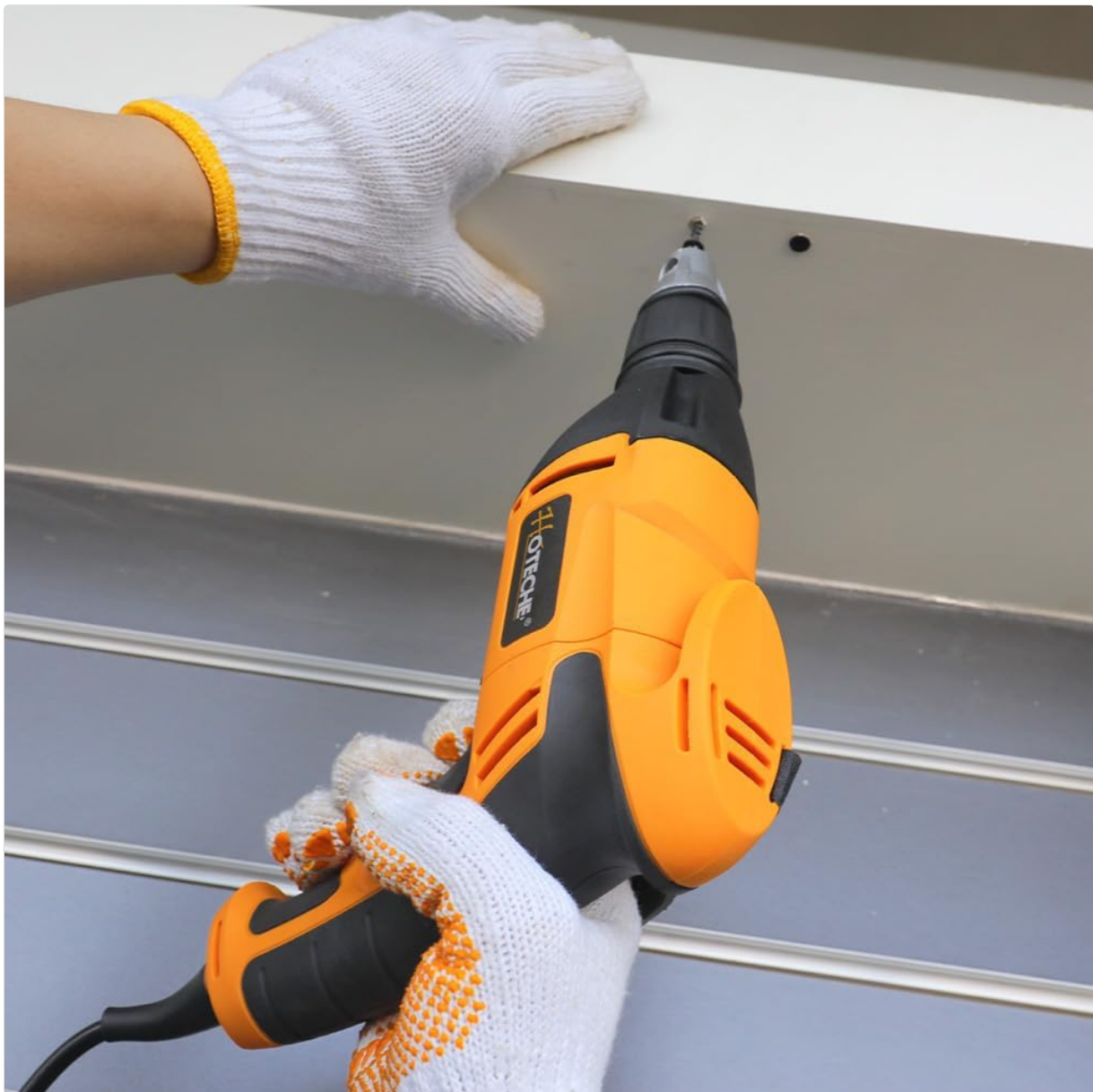
Figure 5.3: Proper technique for driving screws into a surface using the Hoteche Drywall Screw Gun.
