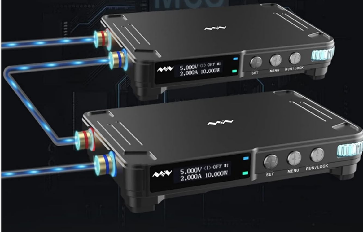
Figure 3: Multiple MDP-P906 units can be configured for series boost or parallel current sharing to meet diverse power needs.
