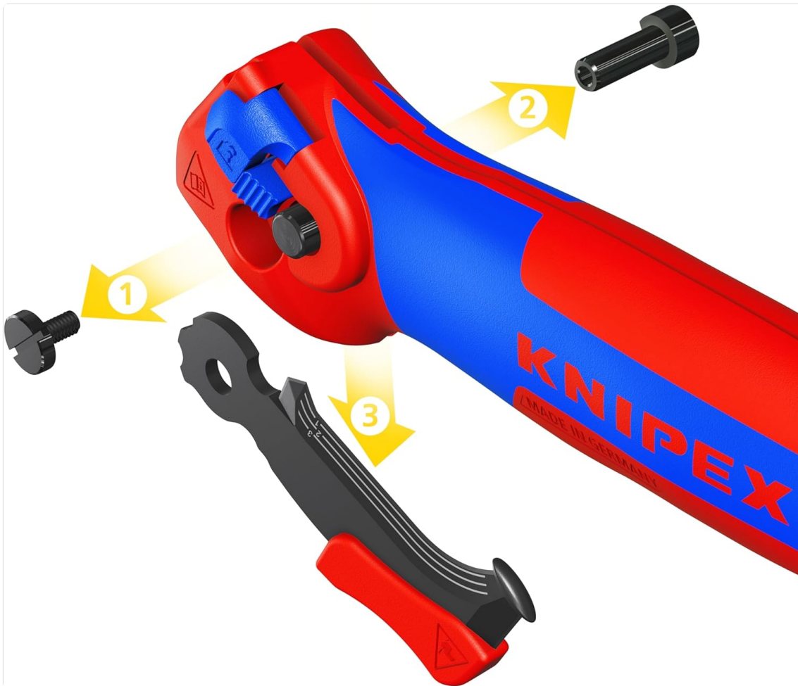
Figure 3: Diagram illustrating blade replacement. (1) Blade retention screw, (2) Pivot screw, (3) Blade assembly.
