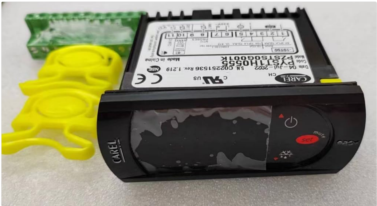
Figure 2: Front view of the temperature controller, illustrating the display and control interface.
