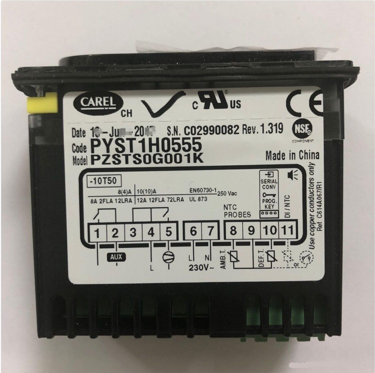
Figure 4: Top view of the controller, displaying the wiring diagram and terminal assignments.
