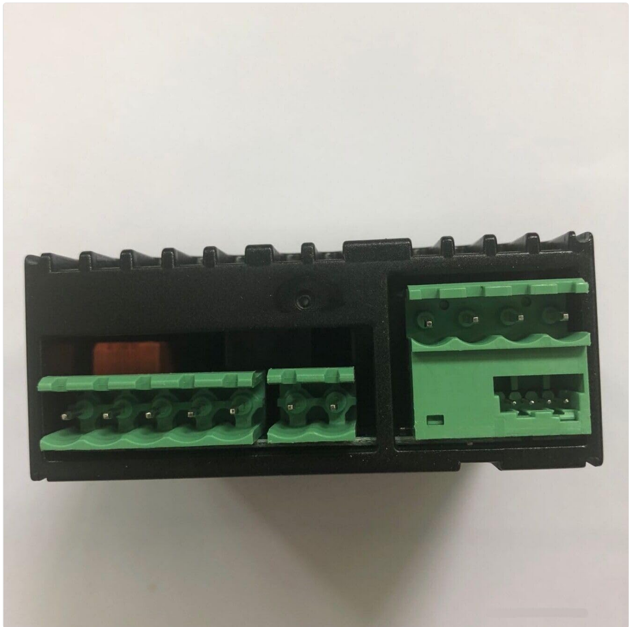
Figure 5: Side view of the controller, showing the connection terminals.
