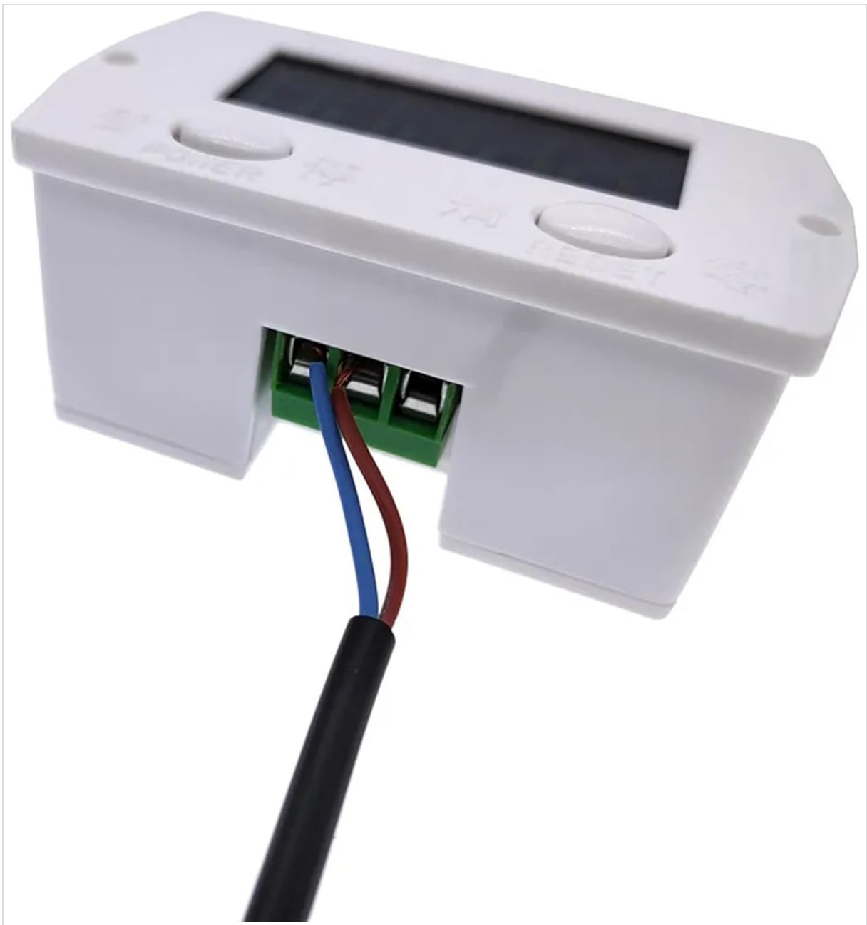
Figure 5.2: Sensor wires connected to the terminal block on the back of the counter.
