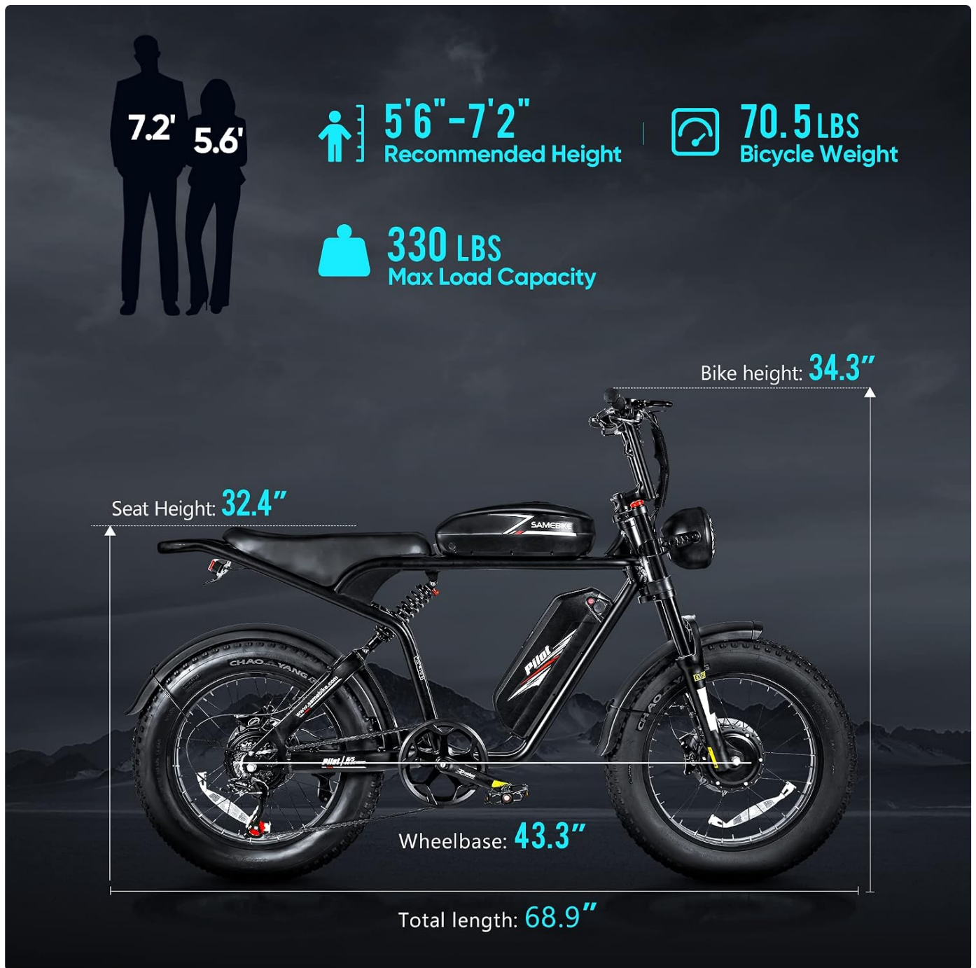
Figure 7: Detailed dimensions of the SAMEBIKE M20, including bike height, seat height, wheelbase, and total length, along with recommended rider height and max load capacity.
