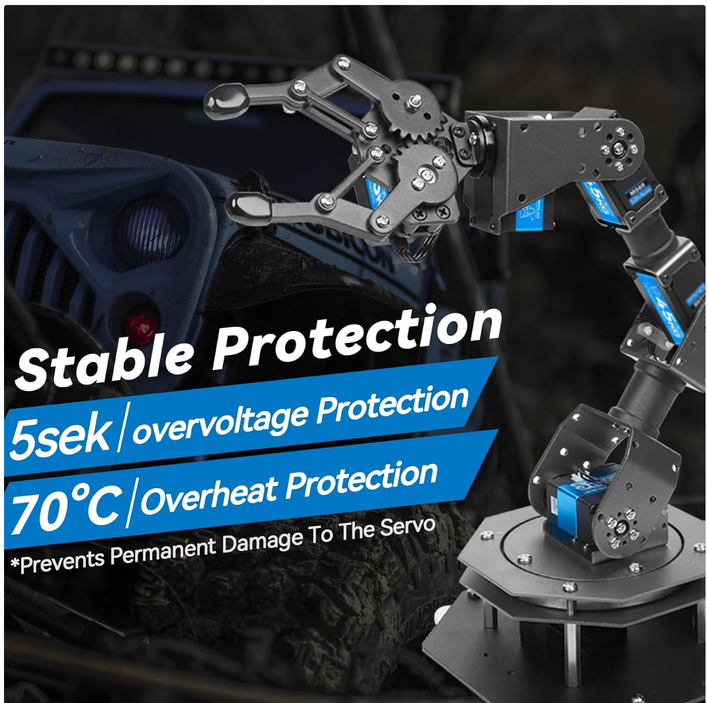
Figure 3: Miuzei 45 kg RC Digital Servo integrated into a robotic arm, illustrating stable protection features like overvoltage and overheat protection.
