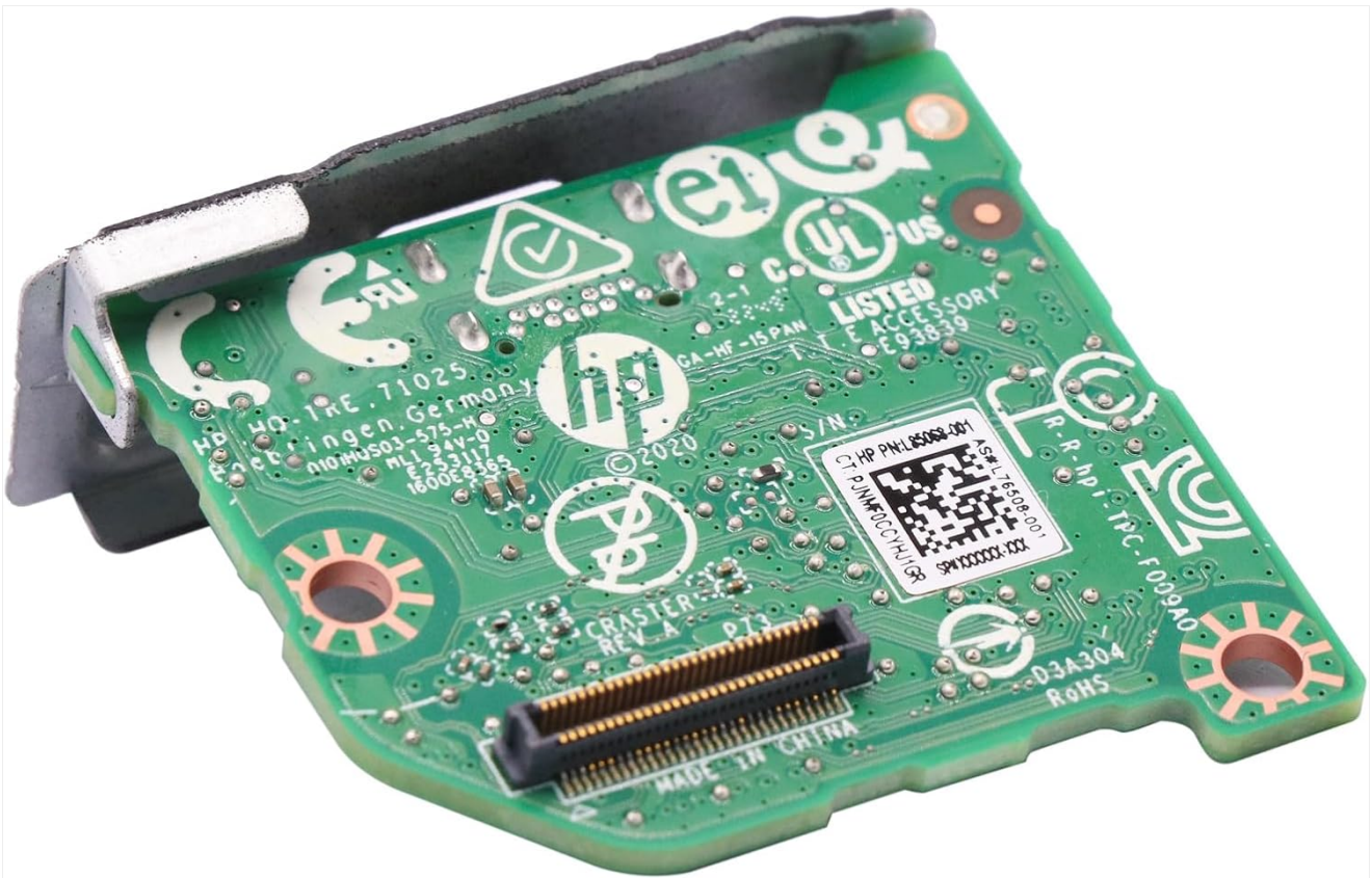
Image 5.1: Bottom view of the Flex IO card, highlighting the connector that interfaces with the motherboard.
