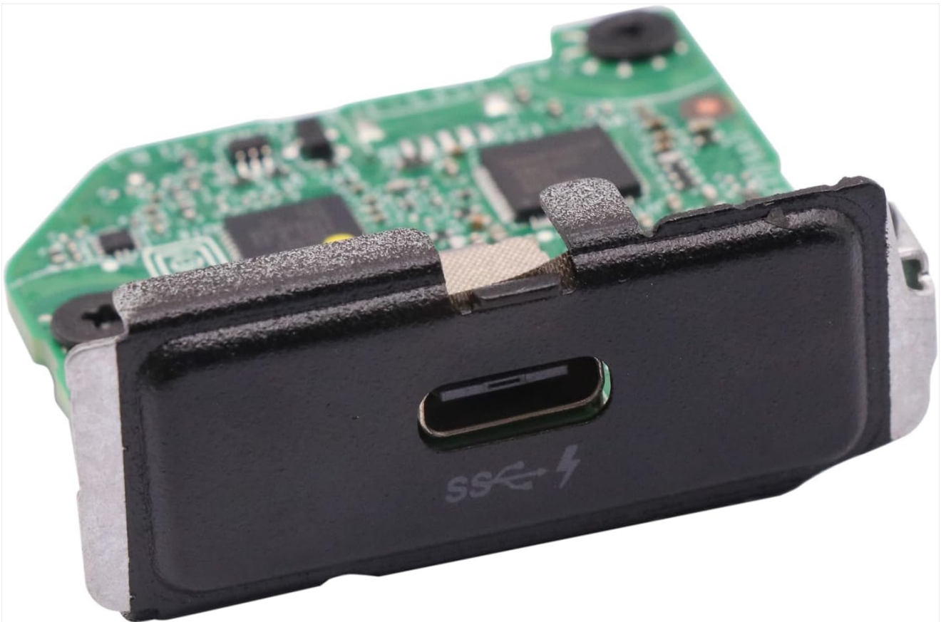
Image 2.2: Close-up view of the USB Type-C port on the Flex IO card, indicating its interface.
