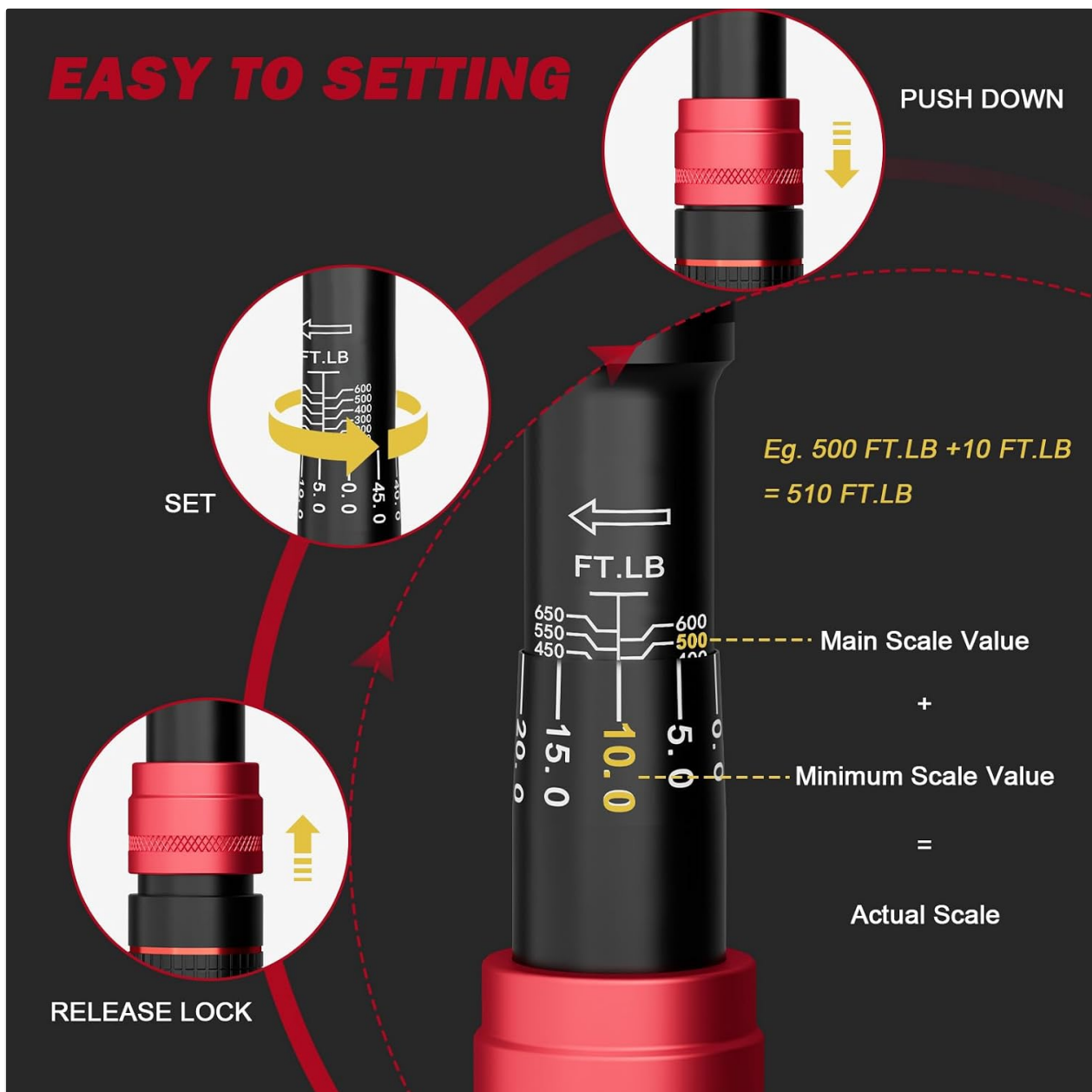
Figure 3: Steps for setting the torque value on the wrench.
