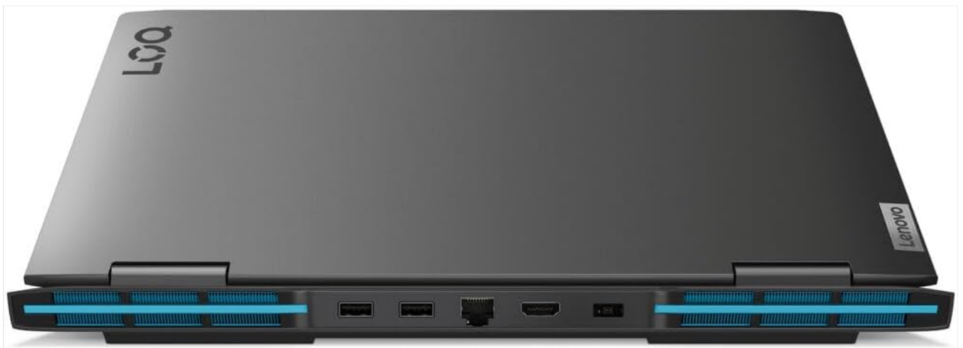
Figure 3: Rear view of the laptop, showing the main cooling vents and power input.
