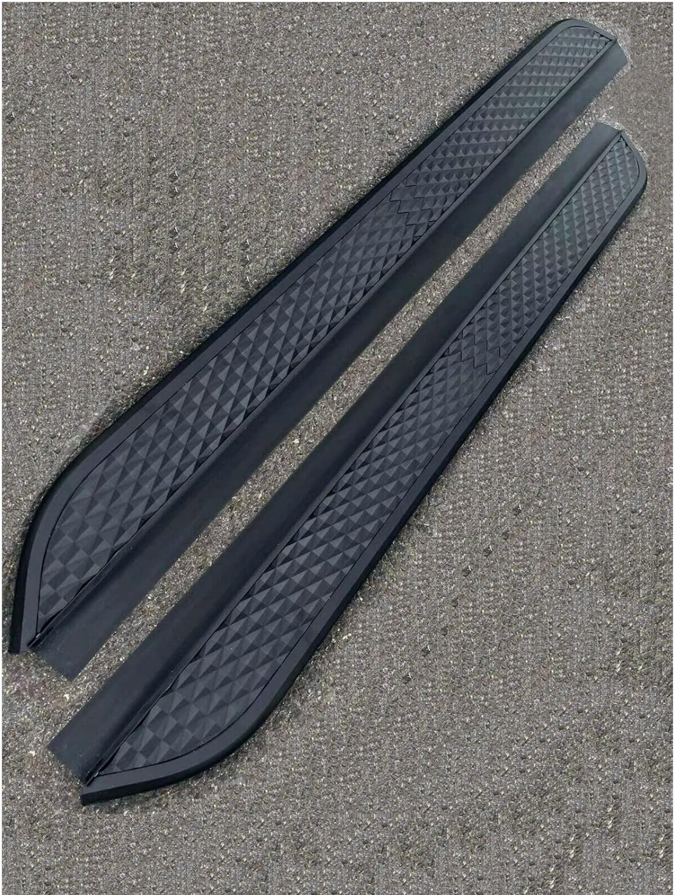
Image: Two running boards showing the textured top surface.
