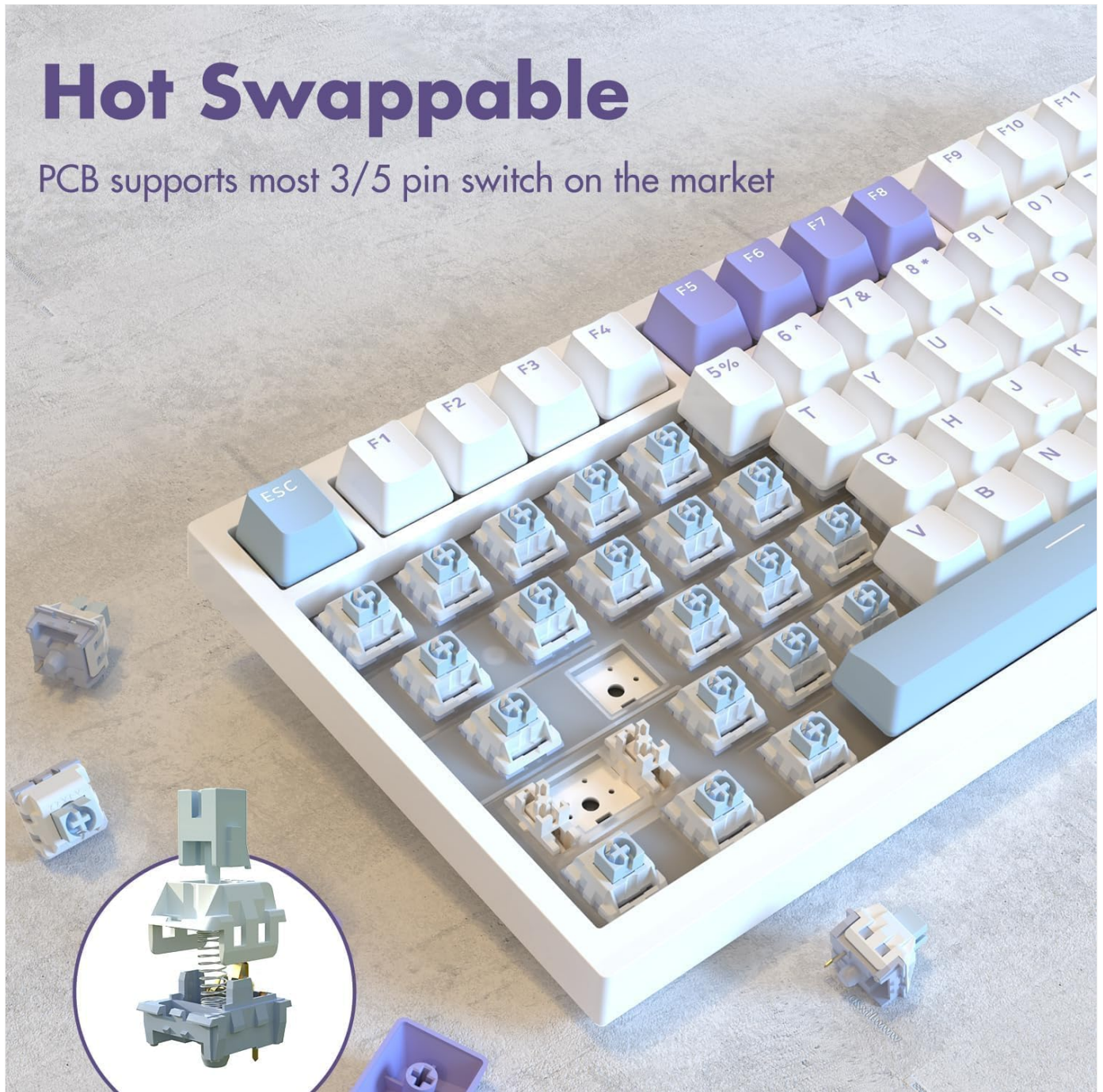
Image 5.3: A section of the AJAZZ AK820 keyboard with several keycaps and switches removed, illustrating the hot-swappable PCB feature. Individual switches and their components are also shown.
