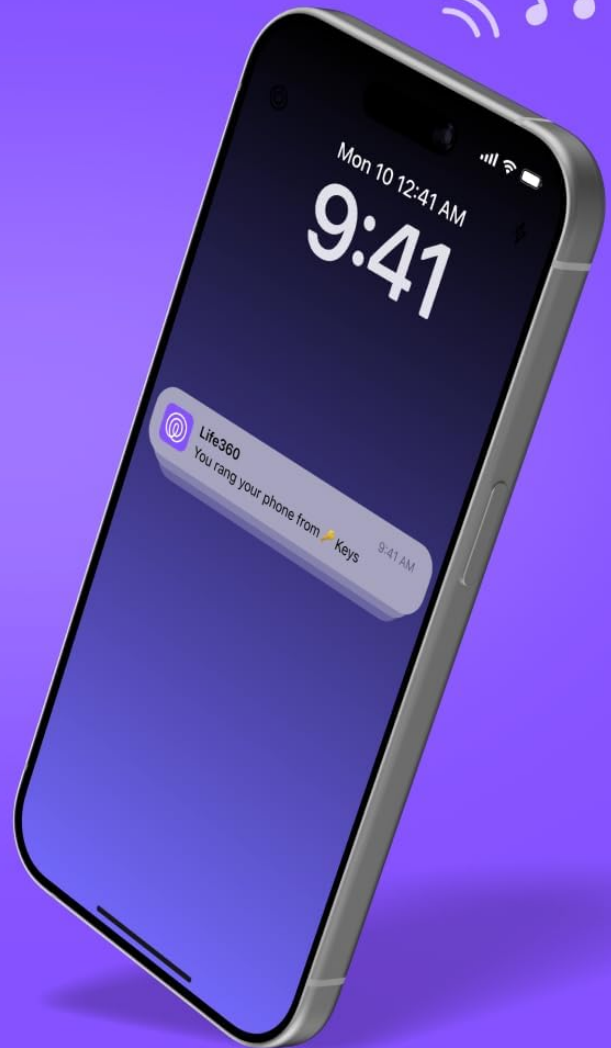
Image 4.2: Using the Tile Sticker to ring a misplaced phone. A double-press on the Tile button activates this feature.
