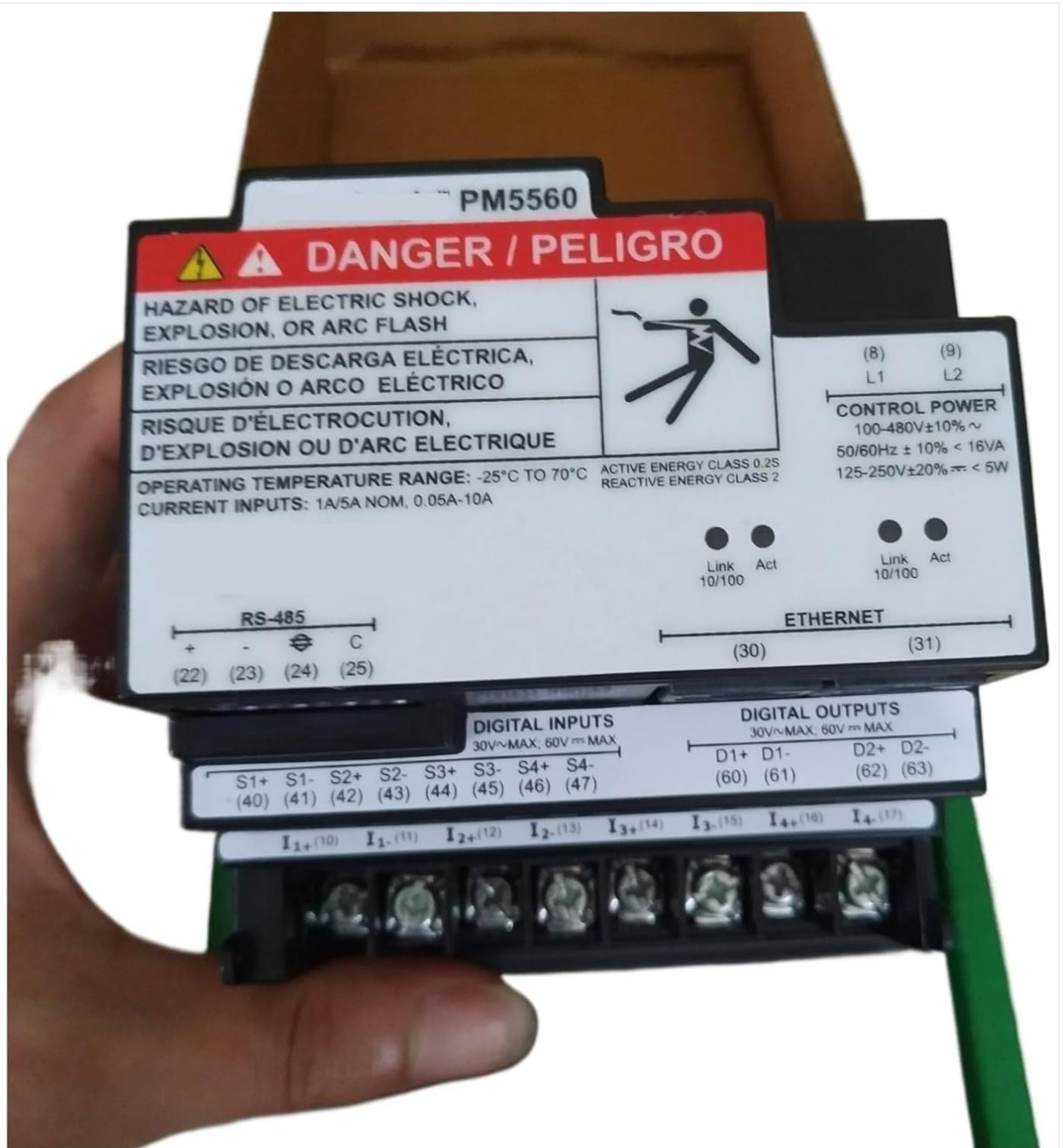
Figure 1: METSEPM5560 Power Meter showing safety warnings and connection points.
