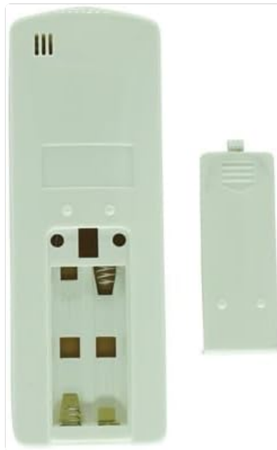
Image: Back of the remote control with the battery compartment open. This image illustrates the correct orientation for inserting two AAA batteries into the remote control.
