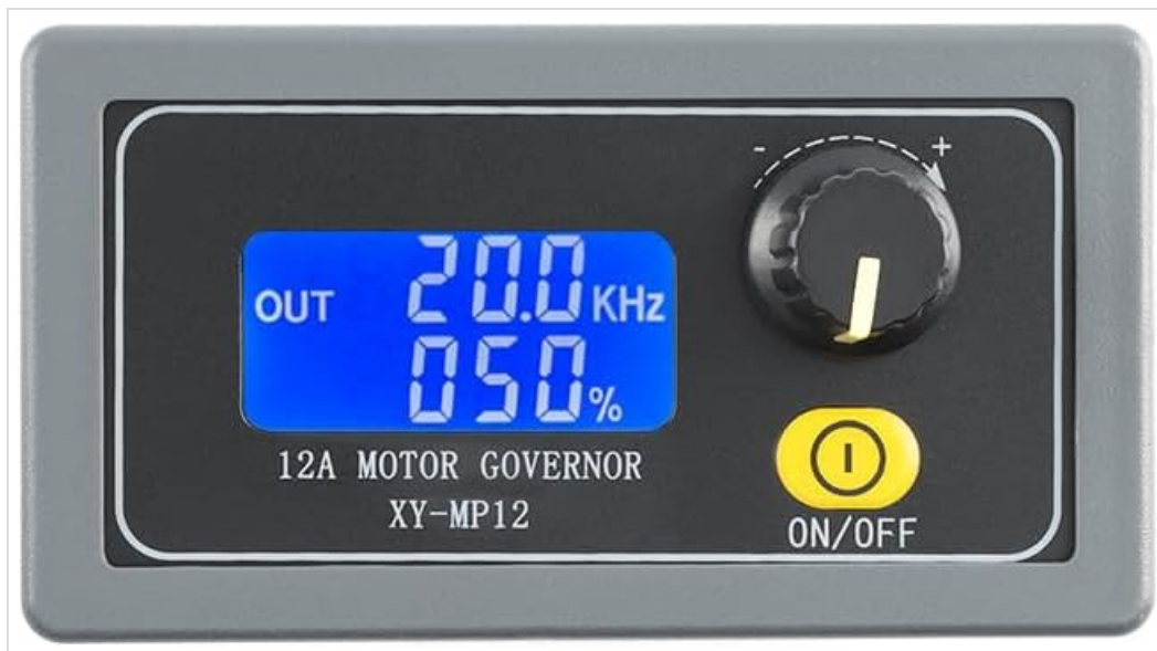
Figure 2.2: Front panel of the XY-MP12-W controller, displaying the LCD screen for frequency and duty cycle, the rotary encoder, and the power button.
