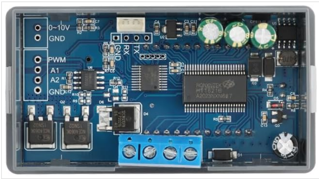
Figure 2.3: Internal view of the controller's circuit board, showing connection terminals for power input, PWM output, and analog control.
