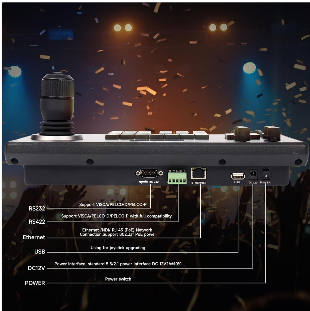
Figure 5.3: KB200 Controller Rear Connections. This image details the rear panel of the KB200 controller, labeling ports such as RS232, RS422, Ethernet (RJ-45 PoE), USB (for upgrading), DC12V power interface, and the power switch.
