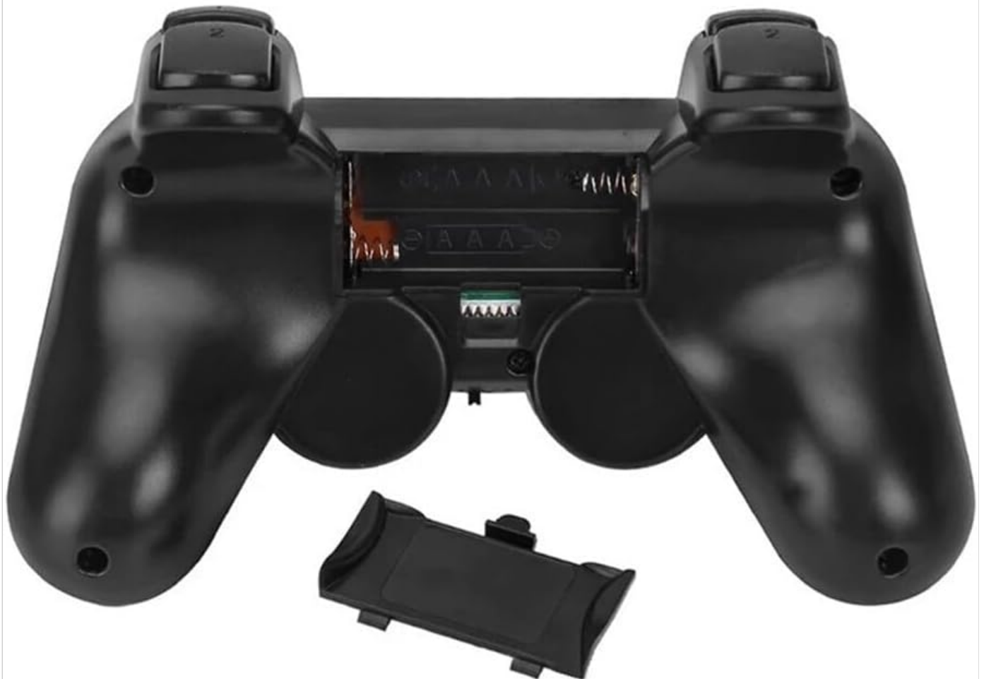
Image: The underside of a wireless controller with the battery cover removed, indicating the placement for four AAA batteries (two per controller) for power.
