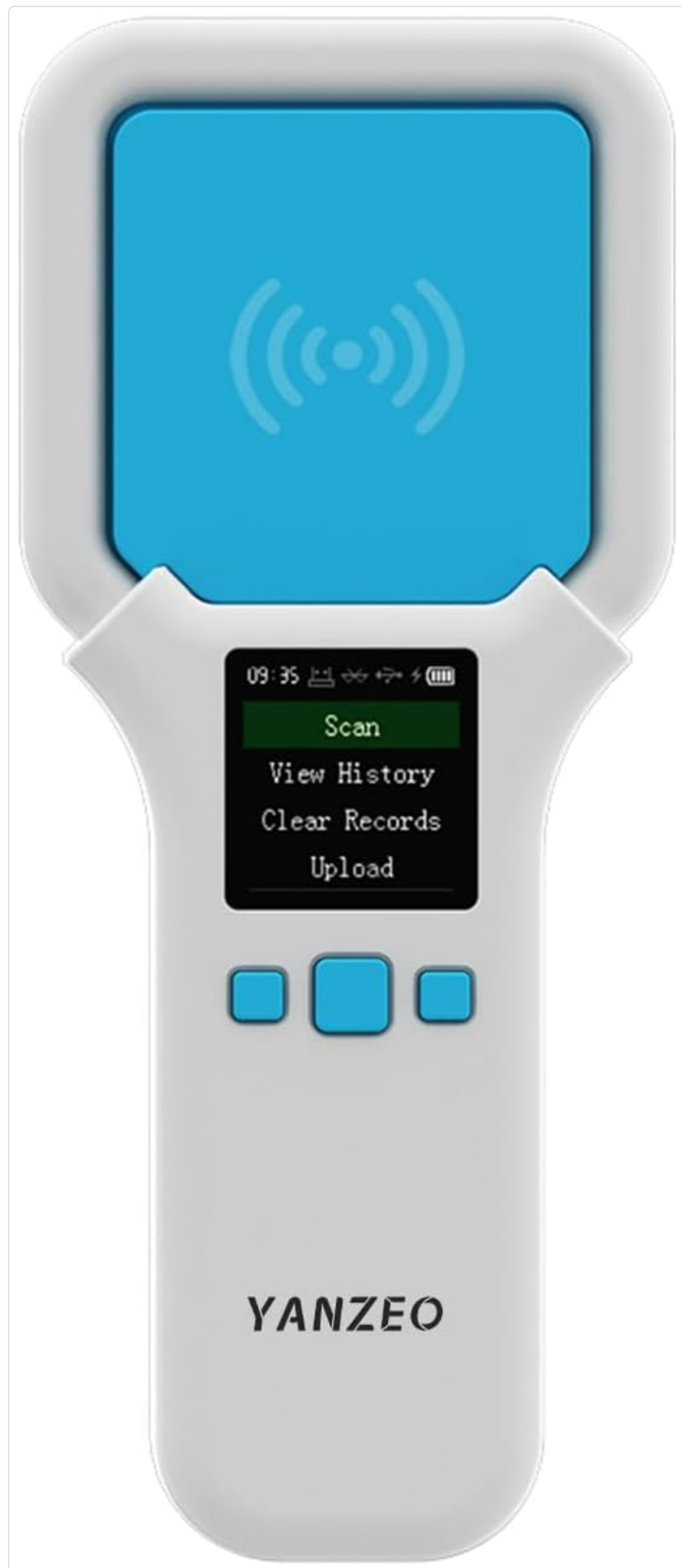
Figure 1: Front view of the YANZEO SR300 UHF RFID Reader, showing its display and control buttons.
